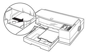
You can load up to 100 sheets of plain bond paper, but do not load paper above the arrow mark on the left edge guide.
